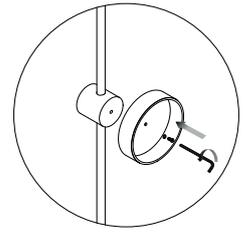
Mount and thread the rear of the central box using the screw and washer provided.
