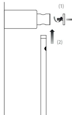
First, unscrew the cap from the anchor (1), second, insert the wooden rod until the marked position (2), and finally screw the cap again until the clock is properly fixed (3).
